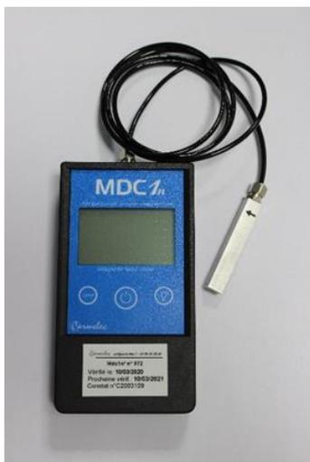
MDC1n<sup>2</sup> is a device for measuring tangential fields.
